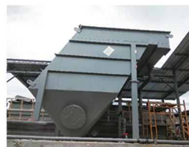
3. Model: XBC-60 Capacity: 60m 3 /h Wastewater type: chicken slaughterhouse wastewater Location: Malaysia
