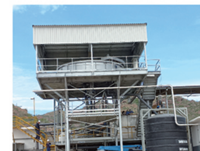
4. Model: GQF-70 Capacity: 70m 3 /h Wastewater type: paper-making wastewater Location: Mexico
